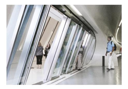
Inclined sliding doors record PST 20 installed at this transport terminal in Germany
